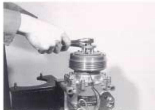
Fig 1. Removal of Armature Fixing Nut
