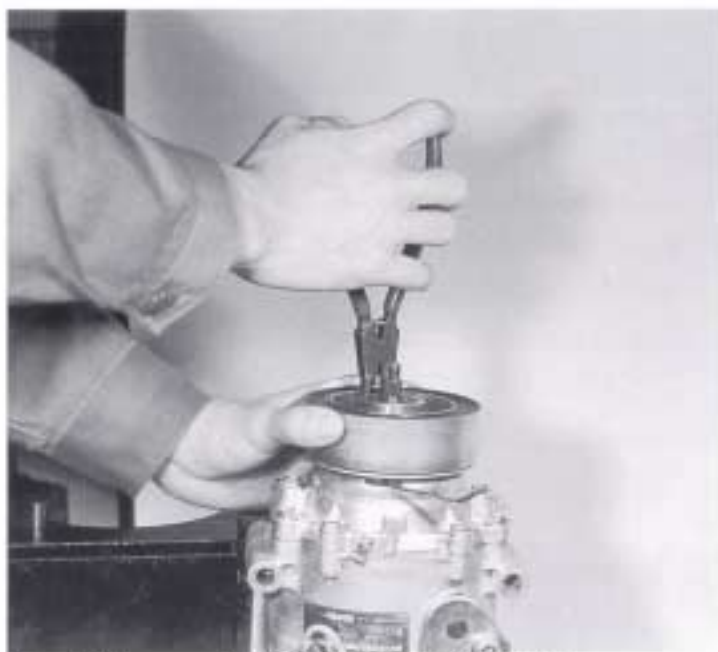
Fig 5. Removal of Clutch Coil Assembly
