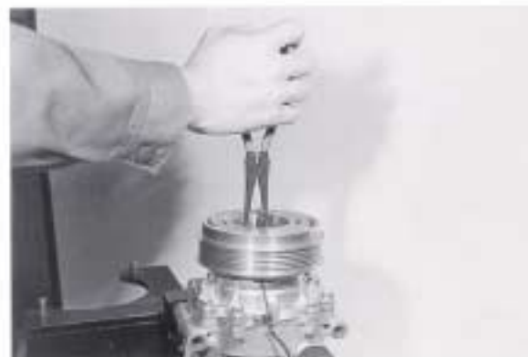
Fig 8. Installation of Snap Ring
