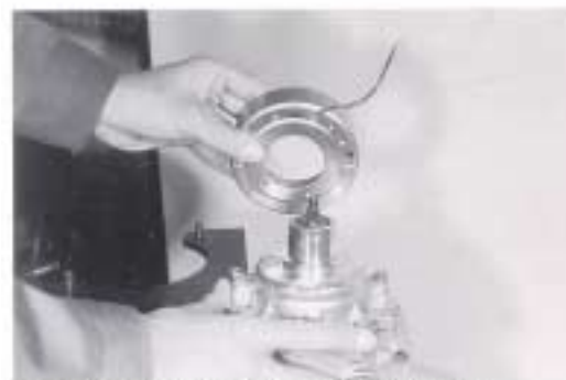
Fig 6. Installation of Clutch Coil Assembly
