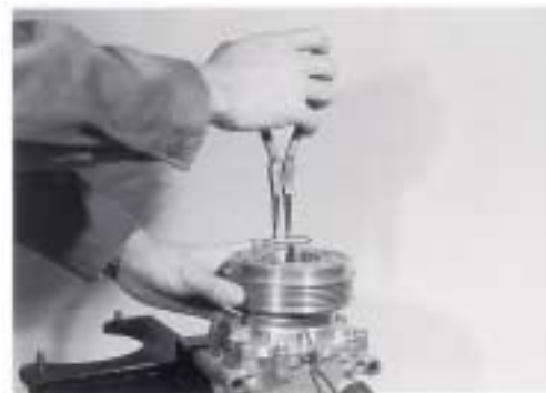
Fig 3. Removal of Snap Ring
