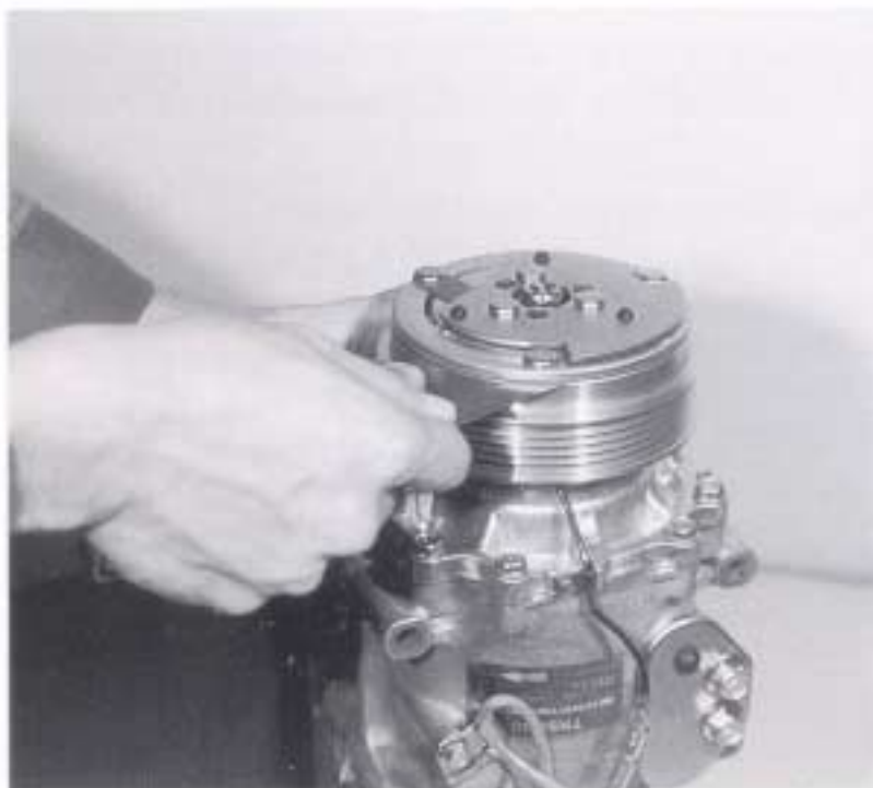
Fig 10. Air Gap Adjustment
